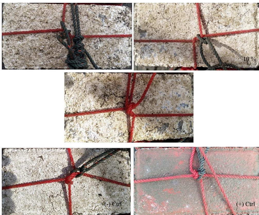
Figure 5. Display of paving blocks with different treatments after 14 days of subtidal immersion.
