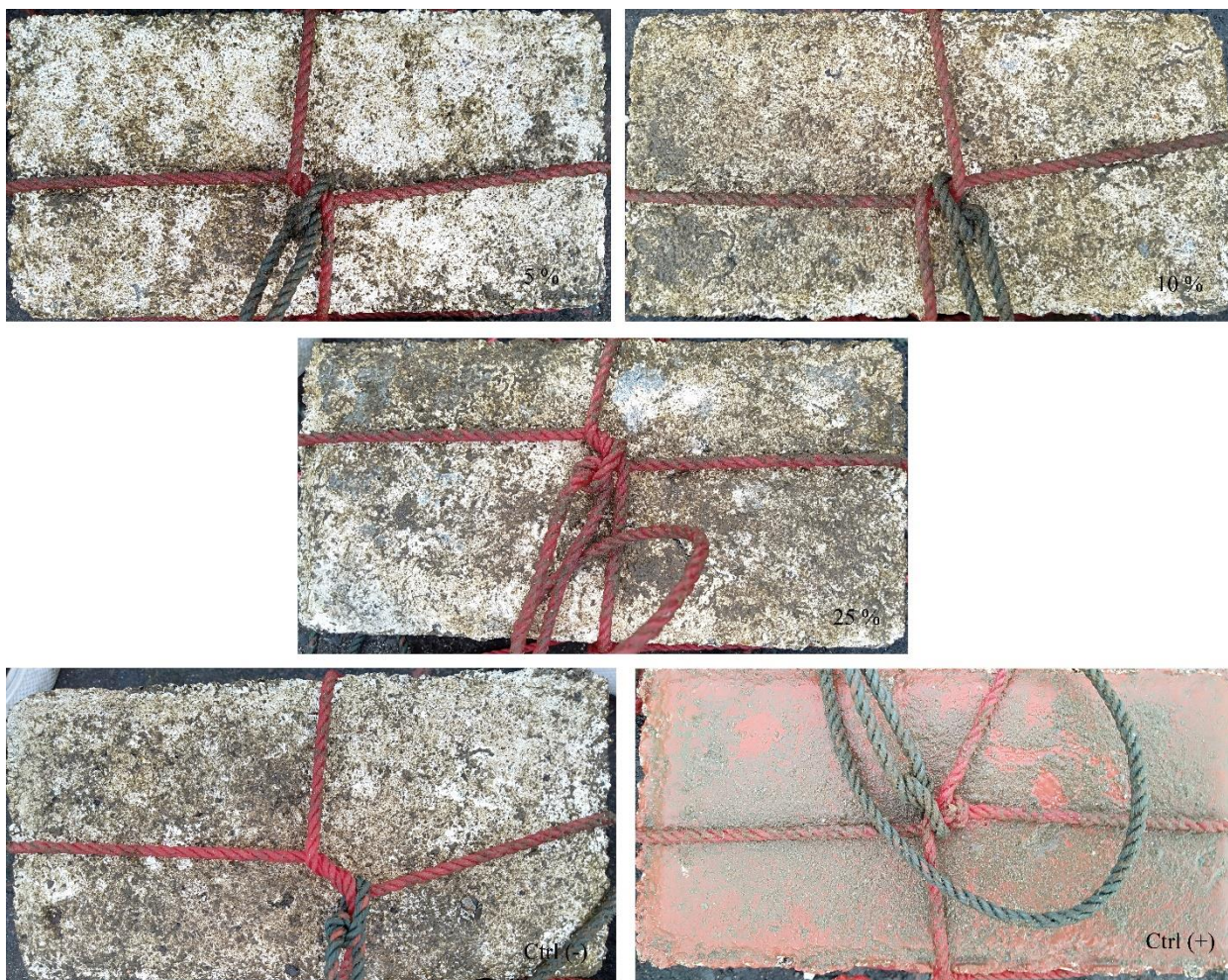
Figure 8. Display of paving blocks with different treatments after 28 days of subtidal immersion.
