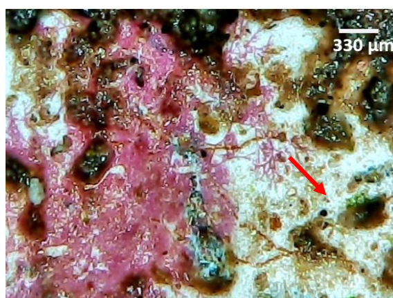
Figure 11. Microscopic appearance of the surface of negative control paving block after 90 days of subtidal immersion
