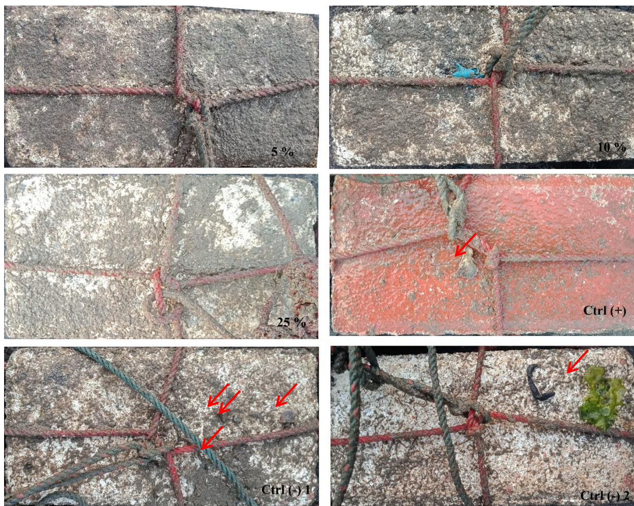
Figure 10. Display of paving blocks with different treatments after 90 days of subtidal immersion. Note Red arrows = macro-fouling organisms.
